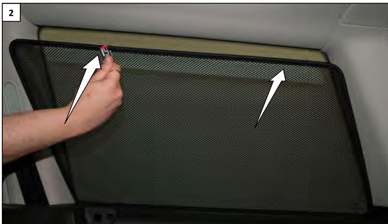
Position shade into place. No fixing clips required
