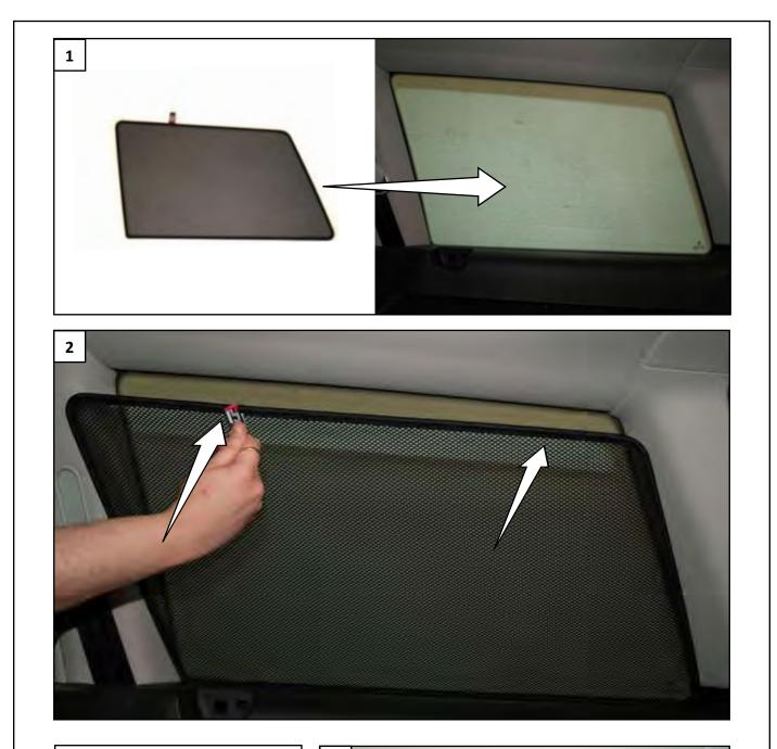
Position shade into place. No fixing clips required
